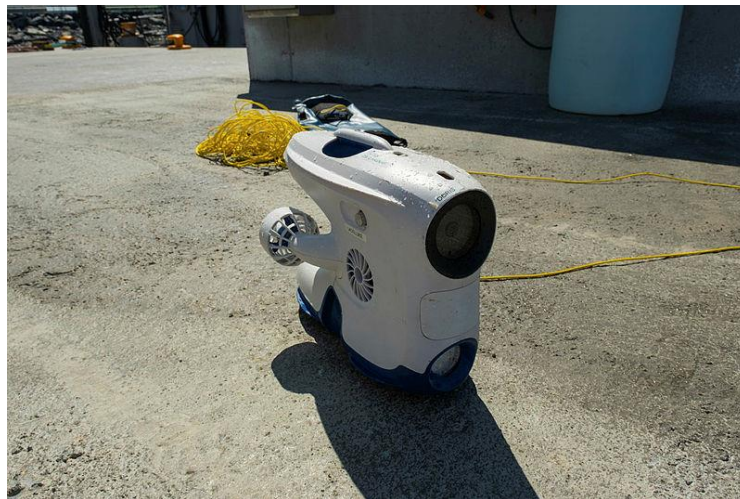
Figur 2: Undervannsdronen Blueye Pioneer.
